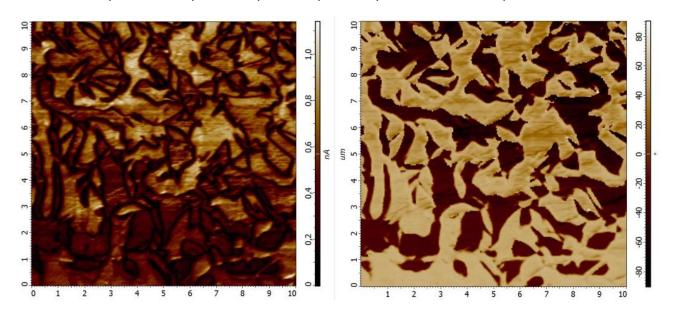
The same scan area after polarization by voltage -10 and +10 V in PFM mode
