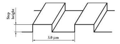
Step height is the average meaning based on the measurements of 5 gratings with the same height (from the batch of 300 gratings) by AFM calibrated wih help of PTB certified grating TGZ1. Basic step height can vary from the specified one within  $\pm 10$  % depending on the batch (for example TGZ1 grating can have step height  $22\pm 1.5$  nm).
