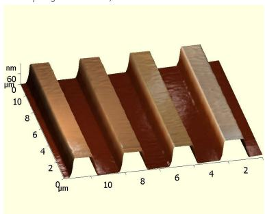
AFM image of TGZ1 grating (step height 20nm).
